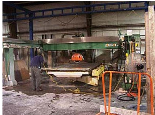
*Cutting in the shop is completed using one of three bridge saws, including one manufactured by Pedrini of Italy.*
